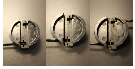
3. It is always a good idea to saturate the area where the splice and piercing pins are with Marine axle grease. This can be found at any Auto parts store in the axle grease section. This will eliminate future corrosion and connection problems.
