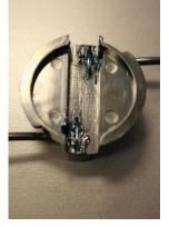
4. Insert your 12 Awg landscape lighting cable into the slot and press straight down on the piercing pins. Make sure the pins have pierced straight into the cable where the copper is located to insure good contact. If the landscape lighting cable is inserted at an angle the brass pins may bend. If this happens straighten the brass pins out with a pair of needle nose pliers and re-insert the cable. Lock the cap back on and test your connection.
