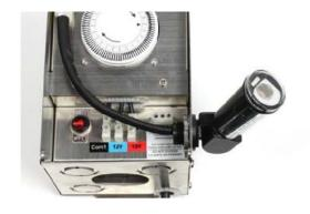
Plug the photo cell into the now empty socket connection.
